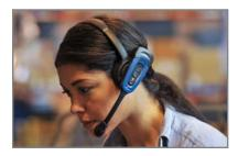
The SRX2 wireless headset provides an embedded multi-microphone array to reduce unwanted word and sound insertions by more than 50% compared to other headsets used in the distribution center. It uses high fidelity acoustic sampling for higher audio clarity.
