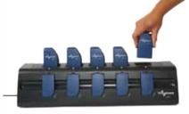
The T1 Voice Appliance easily slips into and out of the charger. There is no need to remove its battery; workers in a hurry can simply drop the T1 in for a charge. However, there is also a slot in the front of each terminal charging bay to charge an additional battery for longer shifts or back-to-back shift operations.
