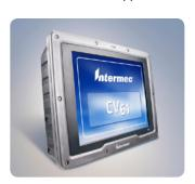
performance while making it easy to upgrade from legacy vehicle-mount systems. Running either Windows 7 Professional or Windows XP, the CV61 includes a 30.7 cm (12.1 in) LED-backlit touchscreen display, 1.8 GHz Intel Atom processor, an IP66 rating, and backward compatibility with CV60 peripherals.
