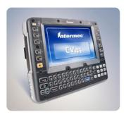
voice systems with Intermec data collection technologies. The CV41 runs the Microsoft Windows CE 6.0 operating system, has an 8-inch WVGA touchscreen display, full keypad and provides VT220, 3270 and 5250 terminal emulation. The CV41 has native support for bar code, RFID and voice input, includes USB, RS-232, headset and other interface ports, plus Bluetooth,
