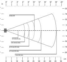
\* The reading distances for each scanner are typical distances measured from the front end of the scanner bezel in an office environment (200 lux) with extended reading range activated.
