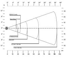
\* The reading distances for each scanner are typical distances measured from the front end of the scanner bezel in an office environment (200 lux) with extended reading range activated.
