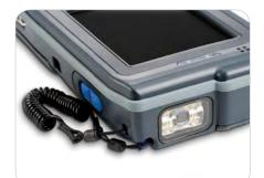
In addition, the Intermec CN3 comes with a built-in barcode scanner, which the consumer-grade devices did not possess. This greatly benefits the engineers, who can scan the set top boxes which they are installing in order to automatically record which version of the product is in a customer's home. Not only does the scanner save time but it also increases accuracy since errors are prone to occur when manually inputting a barcode sequence.
